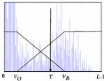
Figure 1. Histogram of a sample image and fuzzy sets  $O$  and  $B$  corresponding to gray level  $T$  as the threshold.
